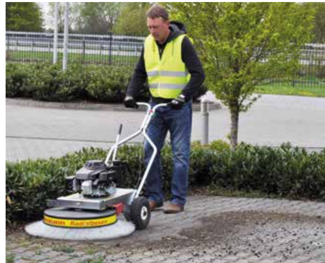
Equipped with a wire brush, green growth is ideally removed even in narrow passages.
